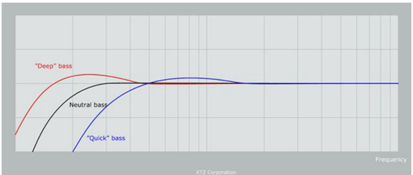
This schematic picture (which does not show actual measured curves) elucidates the different sonic characteristics of the bass frequencies.
